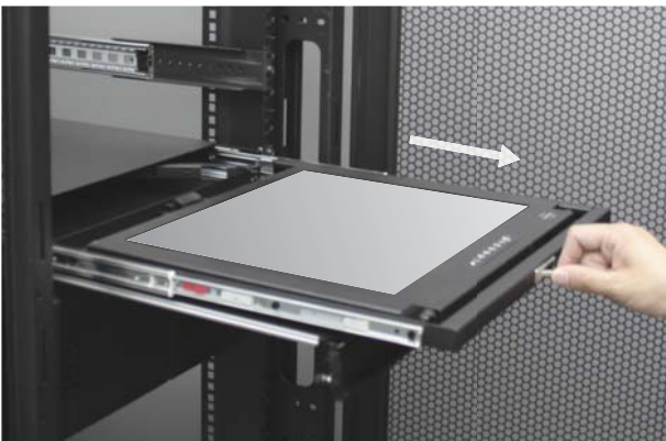
Figure 12. Pulling the handle toward the front of LCD drawer.
