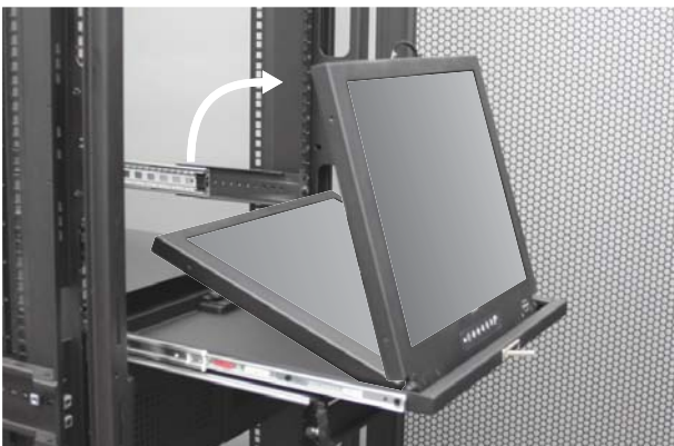
Figure 13. Flipping up the LCD to a suitable angle.
