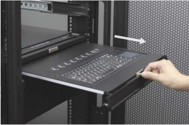
Figure 11. Pulling the handle toward the front of keyboard drawer.
