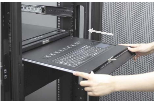
Figure 7. Pushing the lower keyboard drawer into the rack.
