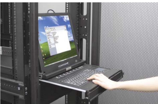
Figure 14. Operating the LCD keyboard drawer.
